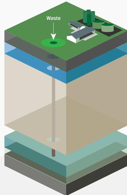
With our patented slurry injection process, liquid waste streams are injected thousands of feet below the water table, permanently sequestering carbon and preventing GHG emissions and ground contamination.
